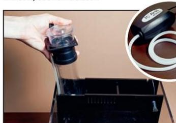
**3** Next place the skimmer in the dedicated chamber, taking care to ensure that it points the right way. Connect the air pump, using the non-return valve in the air line.
